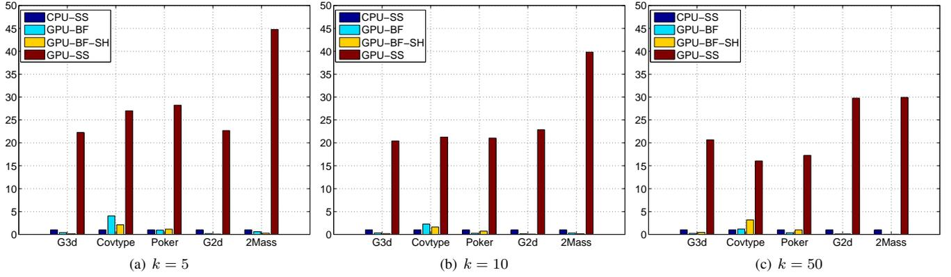
Fig. 7. Speedup over CPU-SS for various values of  $k$ .
