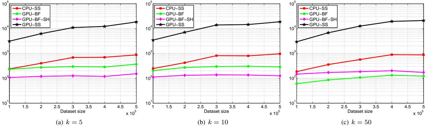
Fig. 6. Speedup over CPU-BF on *G2d* for various values of  $k$ .
